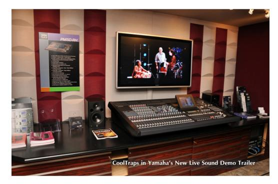
Its design is a curved barrel face with beveled ends. This is not a particularly new shape in the acoustic world but its small size is certainly new. The CoolTrap is only 12" square and just over 3" deep. It is curved in one direction and angled in another. This makes fitting them together into larger and more complicated patterns a breeze. Best of all is that the visual and sonic results from these patterns are simply amazing.
