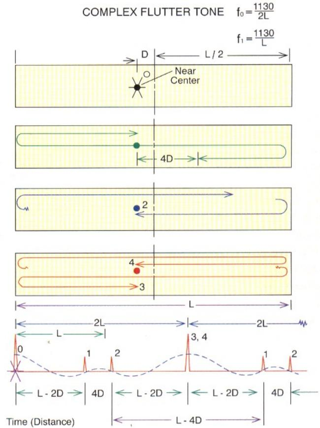
they are essentially all on top of each other. As we move closer to the center of the hall, the timing between the two separate pulses again gets smaller. This time, they do not sandwich and are as far as possible from the double-strength pulse. Finally, at the center, the time between them goes to zero, creating a second, double-strength pulse.
