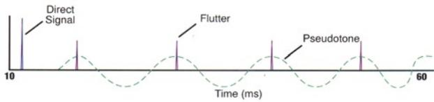
should have been needed. In order to eliminate the detection of a flutter echo pseudotone, we need only to break up the flutter echo process. It takes very little scattering or absorption of high-frequency sounds to break up the flutter echo sequence, and thereby eliminate the accompanying impression of the low-frequency sounds of the flutter tone.
